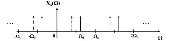
recovered signal after low-pass filtering, with cut-off at  $\Omega_S/2: x_c(t) = \cos[(\Omega_S - \Omega_0)t]$
