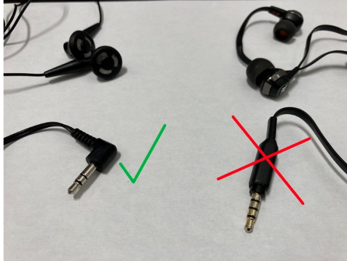
Figure 7: A two ring mini-jack (stereo) should be used.
