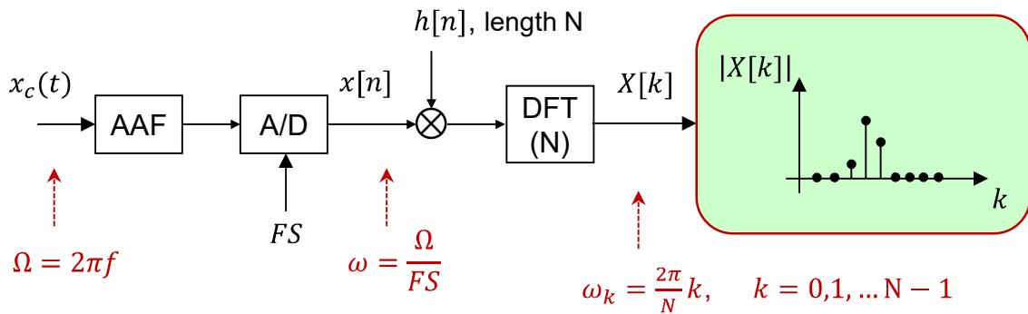
a) In different points of the above signal processing chain, frequency is looked at in different perspectives, i.e. according to different axes as the following scheme illustrates. Explain to your colleagues the correspondence between the three axes (two of them continuous, one of them discrete) and replace the question marks by the correct values (assume that  $FS = 8000 \text{ Hz}$ ).
