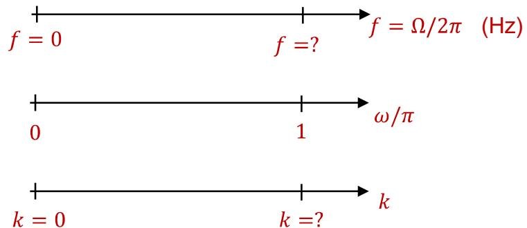
b) The frequency resolution of the DFT is defined as the frequency separation between two consecutive DFT lines (also referred to as DFT bins). If  $FS = 8000 \text{ Hz}$ , and if  $N = 64$ , what is the DFT frequency resolution in Hertz ?
