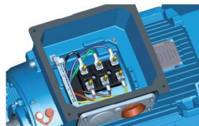
Typical terminal box in motor sizes 71 to 250
