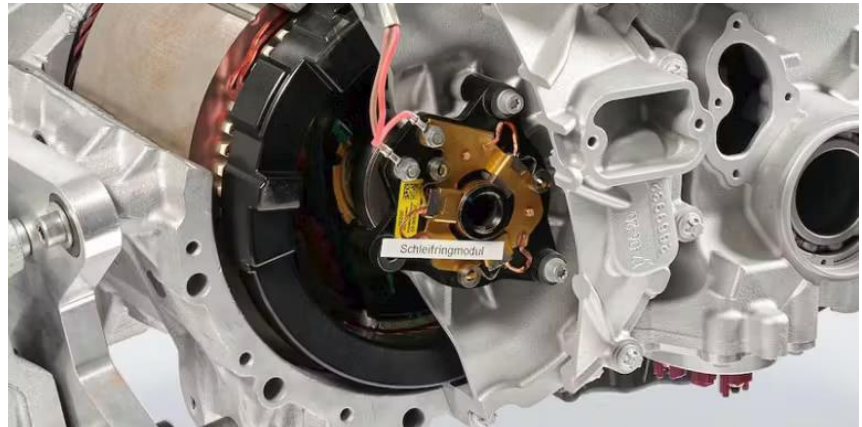
close-up of the slip-ring assembly that powers the rotor of the motor used in BMW's iX-M60 electric SUV Paulo Abreu ®
