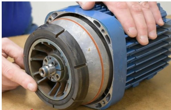
Figure 3 - Demag Conical-Rotor Brake Motor (KB series) using conical friction disk ( ref )
